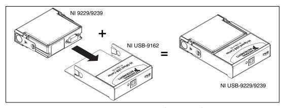
Figure 1. NI USB-9229/9239 Components
